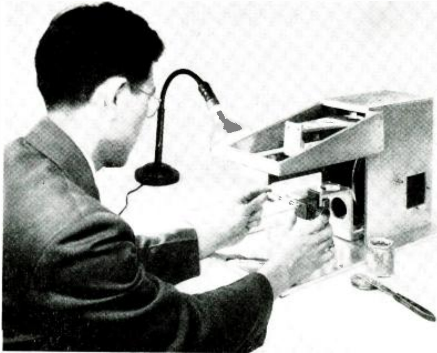
Fig. 5—A specially adapted, inverted rotary press is used to print circuits on cylinders.
