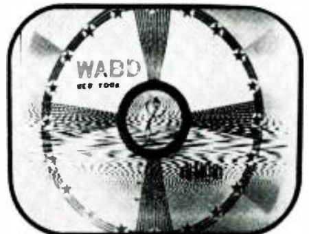
Fig. 5 (above) and Fig. 6 (below)—Diathermy and other devices may bring these bad results.
