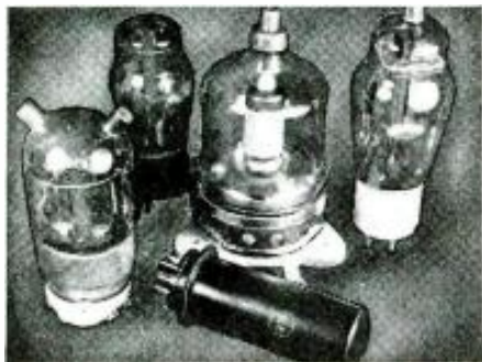
Typical tubes used for class-AB2 modulators.
