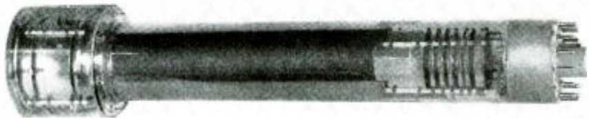
The small size and convenient shape of the image orthicon suit it for many applications.
