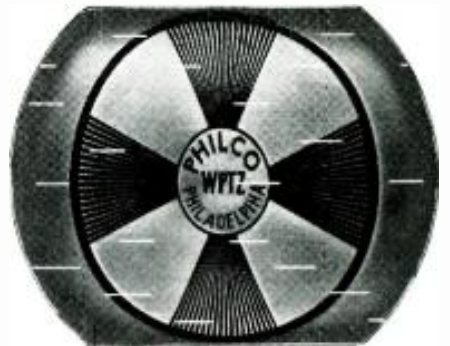
Fig. 4—Moderate ignition-interference lines.
