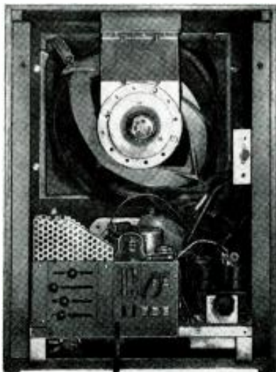
How chassis and tube are set in the cabinet.
