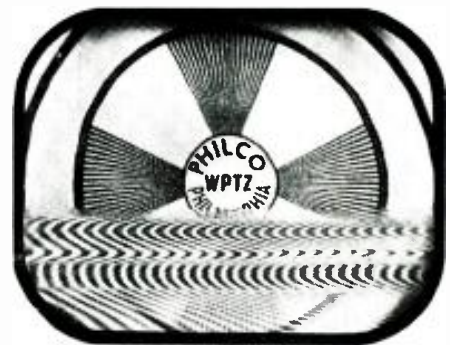
Fig. 5 (above) and Fig. 6 (below)—Diathermy and other devices may bring these bad results.
